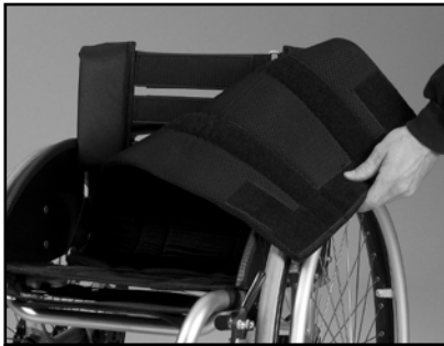
Image 22 Fold the back of the upholstery
