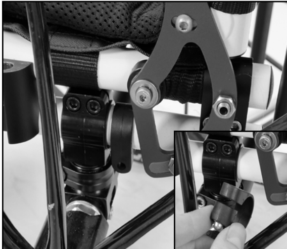
Image 66 Clamp on the frame
