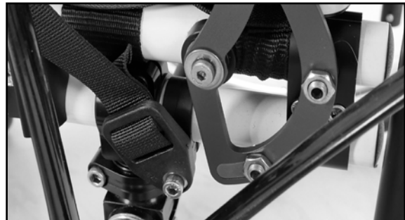
Image 67 Install strap bracket with the bolt
