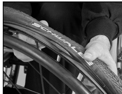
Image 69 Pull out the tube
