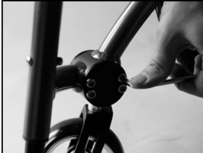
Image 53 Loosen the four bolts
