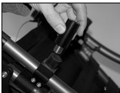
Image 51 Change spacing axle
