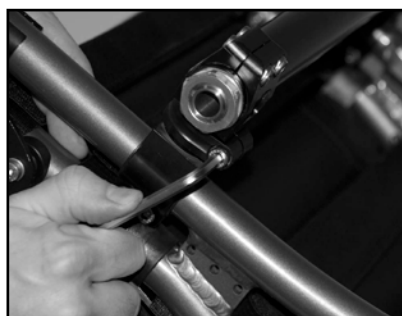
Image 50 Remove the rear axle
