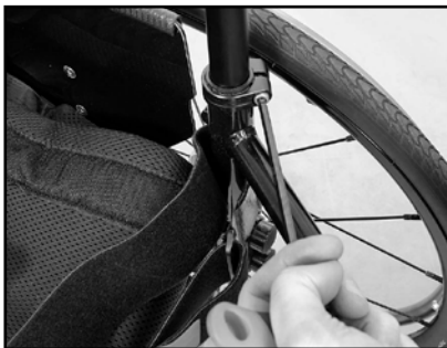
Image 24 Loosen the clamp
