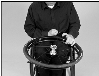
Image 68 Pull the tyre edge over the rim
