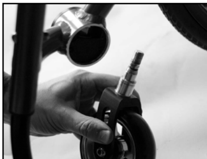
Image 57 Change the caster with front fork
