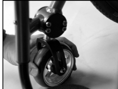
Image 54 Turn the caster + bearing housing
