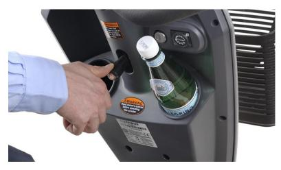
If you'd like to adjust the height of your Vita Lite tiller simply push the adjustment lever down towards the floor until the tiller moves freely up (away from the seat) and down (towards the seat). Once the tiller is in a comfortable position simply let go of the lever.
