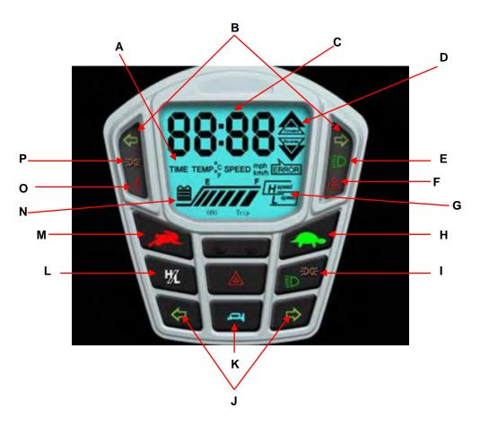
A. **Display Type Indicator** – The relevant light will illuminate indicating that the numerical display (C) above is indicating either time, temperature or speed.
