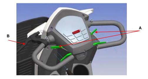
A. **Throttle Controls** – The Throttle Controls adjust the speed of your Vita Lite. The further you pull/push the control the faster your Vita Lite will go.
