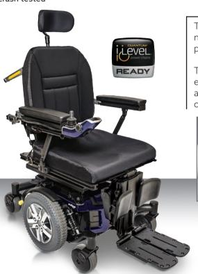
The Q6 Edge® Z Power Chair utilizes powerful 4-pole motors for maximum torque and Mid-Wheel 6® Design for aggressive outdoor performance and precision indoor maneuverability.
