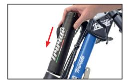
Inserting the Cylindrical battery
