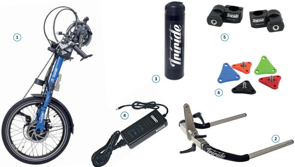
1. Tribike (frame complete with wheel, motor, control unit, steering fork and handlebars with electric controls).
