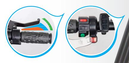
IBS can be used by brake lever or by the electronic brake button that emphasizes the IBS function excluding totally the mechanical brake.
