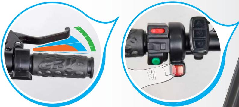
*IBS can be used by brake lever or by the electronic brake button that emphasizes the IBS function excluding totally the mechanical brake.*
