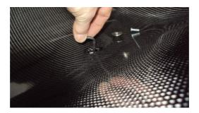
On some 19" models (only) you will need to remove the sealing plug and access the spare wheel retaining screw from above.
