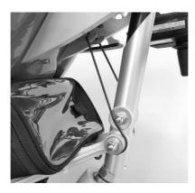
6. Holding the chair stable (by grabbing the front lip of the seat) push the footplate back up, securing where possible (locking & retracting footplate only). Your K2 should now look as below and is ready to transport!
