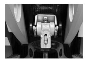
(When replacing this structure, simply reverse the initial movement, squeezing the two plastic buttons on either site and inserting it back into the metal clasp. Occasionally it can twist slightly, so ensure it is straight and fully engaged into the clasp. You should hear a satisfying click when inserted correctly.)
