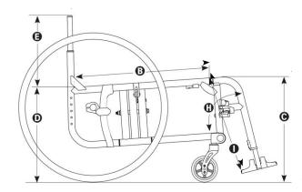
SEAT DEPTH B Measure from 1/2" (1cm) in front of back post to the front edge of seat sling. (12"-14" (30-35.6cm) Seat Depths B not available with 25" (559) and 26" (560) Rear Wheels.)
