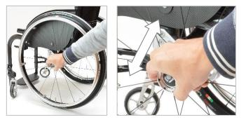
Slightly lift the wheelchair form the ground on one side by holding it on the backrest. Now one rear wheel is not touching the ground.
