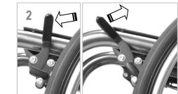
To engage the brake, push the lever forward until it locks.
