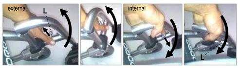
To swing the footplate frame externally, move the lever L sideward to same direction and turn the footplate frame.
