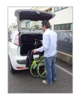
Release the brakes and remove the rear wheels.
