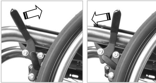
To engage the brake, pull the lever backward until it locks.
