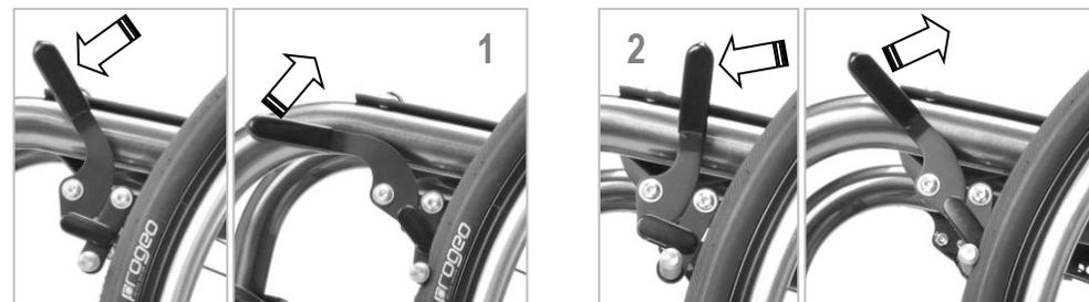
To engage the brake, push the lever forward until it locks.
