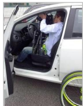
Fold the wheelchair and, with one hand on the front frame and the other hand on the backrest handle to balance the weight of the wheelchair and make lifting it easier, load it into the car.
