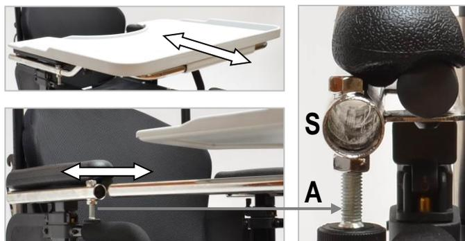
To insert the table, loosen the bolt **A** of the support **S** on each side of the wheelchair until the hole is free to let the tube go through. Insert the tubes parallel into the supports and slide the table to the desired depth. Finally, tighten the bolt **A** of both support **S**.
