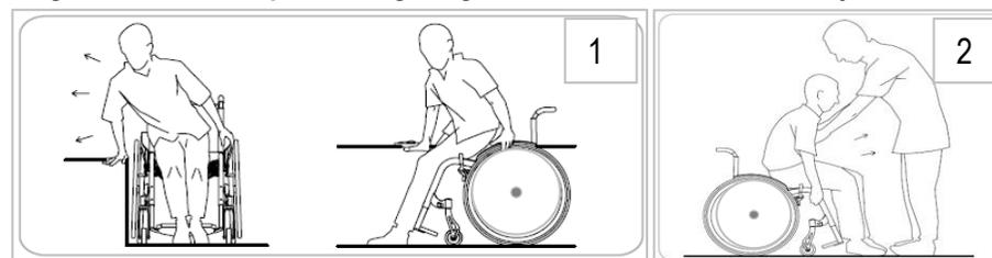
Ensure the wheelchair is parked on a solid, flat or regular surface. Do not get in or out of the wheelchair while on hills or uneven ground which could render the wheelchair unstable and cause the occupant to fall and/or the wheelchair to overbalance. The brakes should be engaged.
