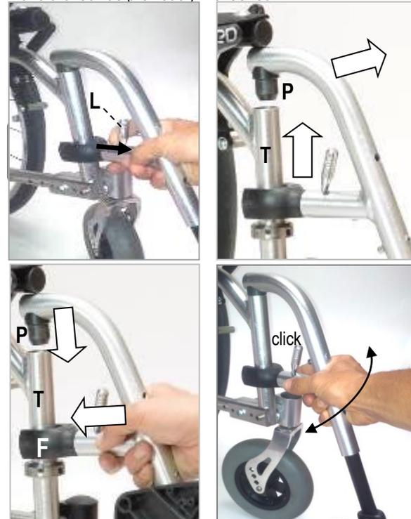
To remove the footplate frame, move the lever L frontward and pull the footplate frame up until the axle P comes out of the tube T. Finally remove the footplate frame.
