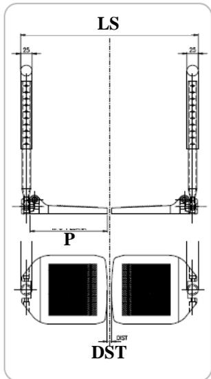
To comply with the rule UNI EN 12183 paragraph 6.1, when double footrests are fitted, it is necessary to maintain the correct distance between the two footrests when lowered:
