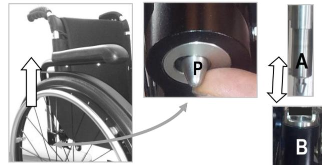
The steel support (made out of the parts **A** and **B**), does not allow the armrest to come off unintentionally. When you pull the armrest up by approximately 1 cm, it should stop at that point. In that position, as above mentioned, you can swing the armrest away.
