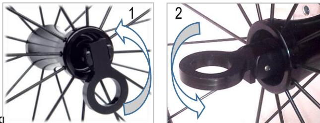
The axle works by turning the ring lever by 90°
