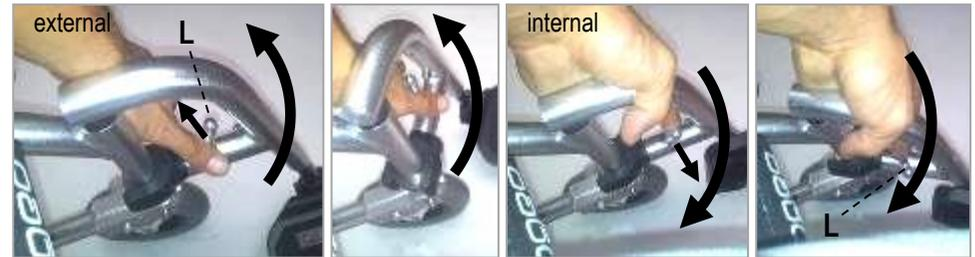
To swing the footplate frame externally, move the lever L sideward to same direction and turn the footplate frame.
