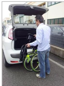
Release the brakes and remove the rear wheels.
