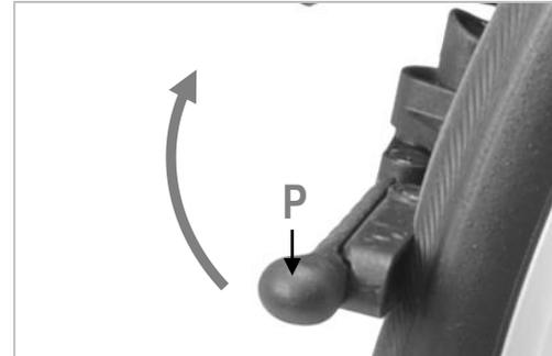
This type of brake reduce the encumbrance of the wheelchair when you remove the rear wheels. It prevents interference with your hand when pushing on the hand rims even with long pushes. On the other hand, in comparison with traditional brakes, its lever is located a lower position and it is less easy to operate. For such reasons, it is not suitable for user with reduced control/movement of the trunk and/or upper limbs and hands.
