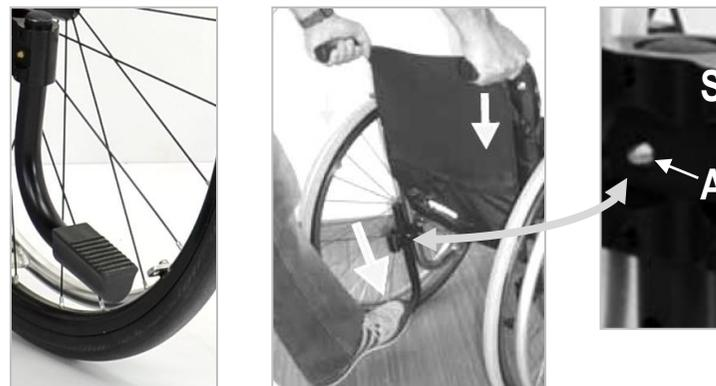
You can remove the tipping aid by pressing the pin **A** that hold it in position and sliding the tube from the support **S**.
