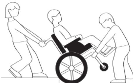
**Figure 3.2:** Assistant positioning for climbing curbs, for wheelchair without step tubes
