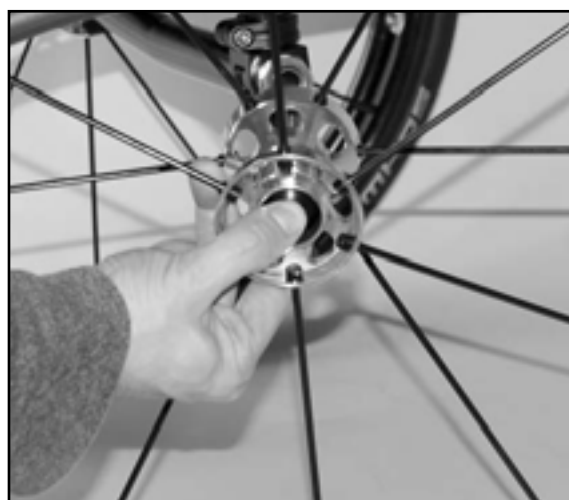
Image 4 Remove rear wheels - QR
