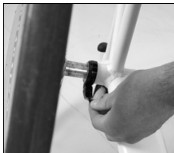
Image 5 Remove rear wheels - W-Rex
