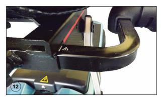
**Warning!** Always check the armrests are locked and secured before attempting to get on or to drive the scooter.
