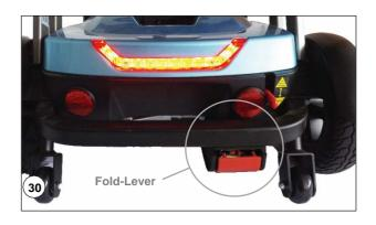
• Take hold of tiller-delta with one-hand, push tiller-delta in a forward direction simultaneously when retracting the fold-lever with the other-hand (Fig.31). This action will dis-engage fold-lock mechanism. The scooter mechanism will then disconnect the internal fold-lock device and then partially un-fold (Fig.32). The support wheels will then be in contact with the ground.
