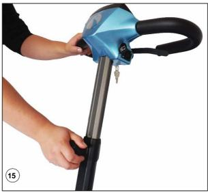
**Warning!** Before driving, always check that the tiller is secured. Safe steering will be impossible if you do not !
