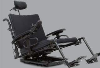
45° of centre of gravity powered tilt.
