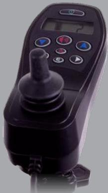
The NE+ controller is a programmable, modular electronic controller system and is available on a wide range of Quantum power chairs.
