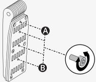
This is how you adjust the height and depth of the headrest.  $\checkmark$  Allen key 5 mm
