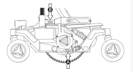
The serial number label is located on the lower, left-hand side of the wheelchair chassis (④). An additional serial number label is located on the seat tilt (⑥). You may need to tilt the seat to see the serial number label.
