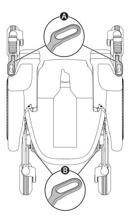
The wheelchair is equipped with four tie-down points used for transportation  $\blacksquare \checkmark \boxdot$ . Two in the front (**(()**) and two in the rear (**(()**).
