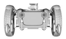
Figure 3. Front Reflectors
