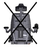
Figure 94. The wheelchair must NOT be fastened by securing it to any part of the seat.
