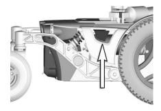
Figure 99. Brake release lever
