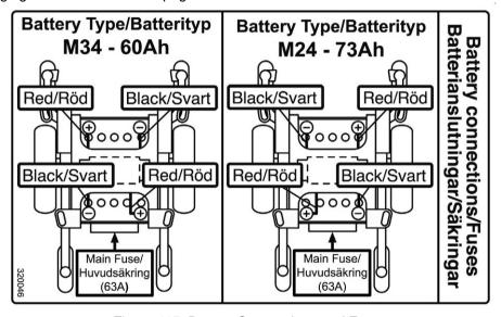
Figure 115. Battery Connections and Fuses.
