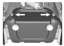
Figure 104. Knobs holding the front cover.
