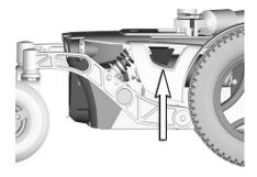
Figure 90. Brake release control.
