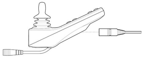
Figure 93. Charging socket on the control panel.
