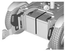
Figure 106. Front battery terminals.
