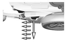
Figure 91. Releasing the brakes
