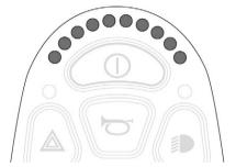
Figure 79. Battery Voltage Indicator
