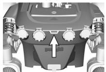
Figure 105. The rear cover is fitted togather with the upper chassis cover.
