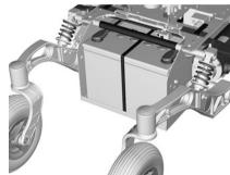
Figure 107. Rear battery terminals
