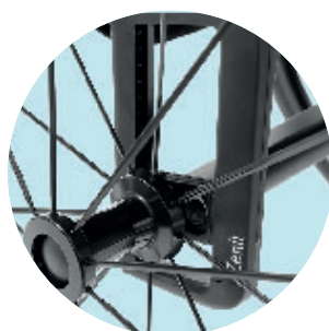
Drive wheel adapter, permanently welded
