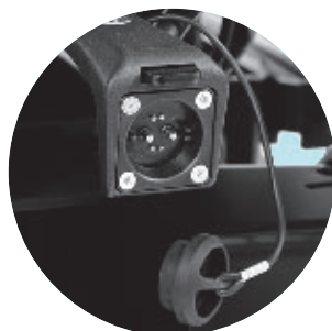
EU043 External magnetic charging receptacle
