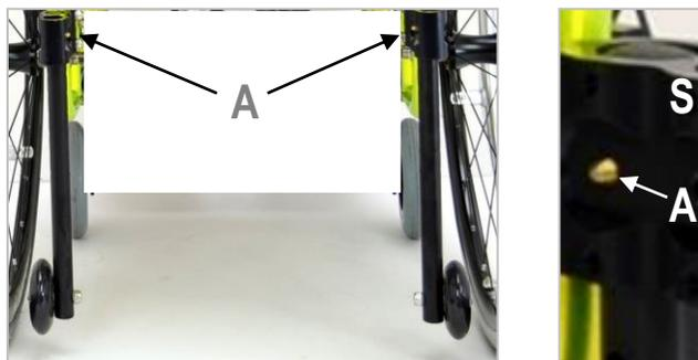
You can remove the transit wheel from its support. Press the pin **A** that holds it and slide the tube off the support **S**.
