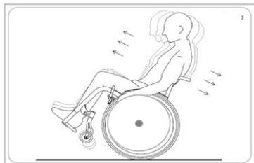
At this point, by moving your body gently backwards and forwards while moving the rear wheel backwards and forwards using the hand rims, it will be possible to find the centre of gravity and the point at which the chair will safely be controlled.
