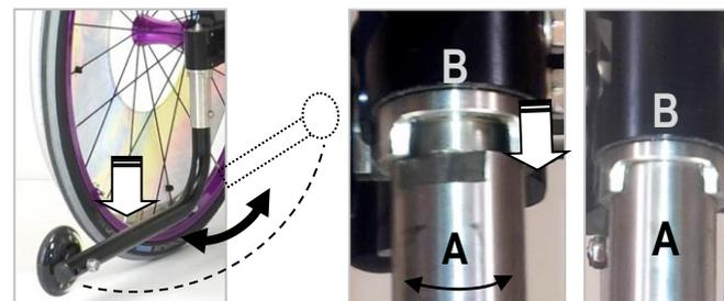
To swing the anti-tip wheel, push it down by approximately 1 cm (the part **A** of the support moves away from the part **B** without coming off) and turn it sideward.
