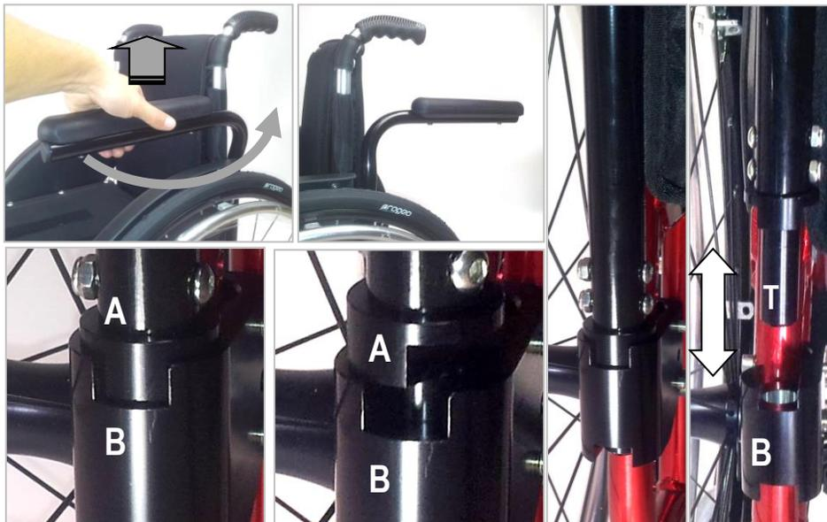
To make transfer easier, you can swing the armrest away on the side. Raise it by approximately 2 cm and swing it away. If wished and possible (the backrest horizontal tube may impeded it), you can swing the armrest away until it locks in its opposite position. To put it back to its using position, swing it in until it locks (if it was locked in its opposite position, raise it by approximately 2 cm first).
