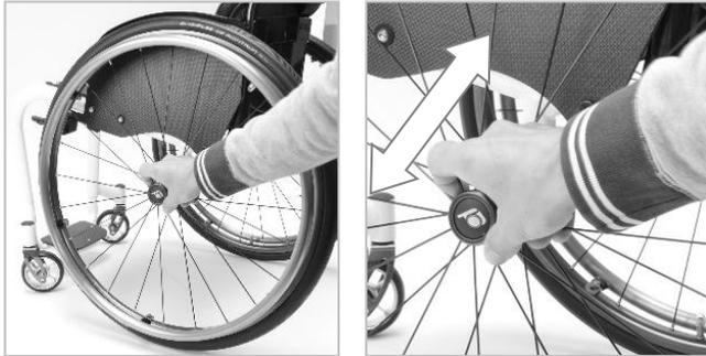
Slightly lift the wheelchair from the ground on one side by holding it on the backrest. Now one rear wheel is not touching the ground.
