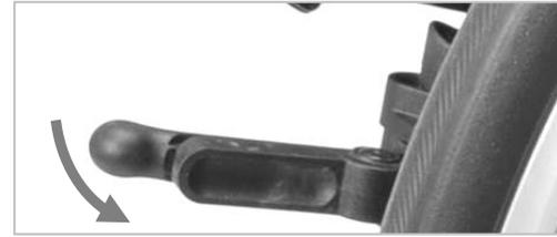
To engage the brake, turn the lever until it locks.
