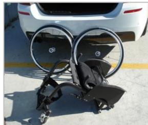
Release the brakes and remove the rear wheels.
