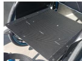
Siti a non-deformable carbon fibre rigid seat board that offer greater stability.
