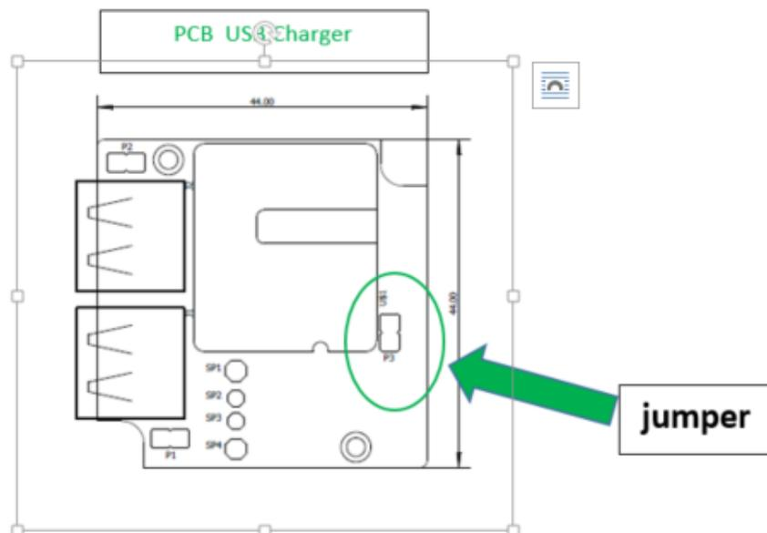
Open the housing of the charger, position the jumper over the 2 pins of the 2 pin header and the charger will work continuously.
