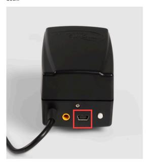
1 Connect the device to a PC. Use a standard mini-USB-USB cable.
