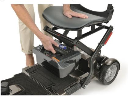
To remove the battery pack of your Minimo Plus first ensure the pack is unlocked by inserting the key into the pack and turning it 90° anti clockwise to the unlock position. Then simply lift the pack up away from the base of the scooter and the seat using the handle provided.
