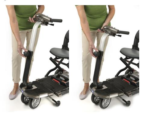
If you'd like to adjust the height of your Minimo Plus tiller simply turn the adjustment wheel anti clockwise until the top part of the tiller moves freely up and down. Then just move the top half of the tiller to the height you would like and tighten the adjustment wheel by turning it clockwise until tight.
