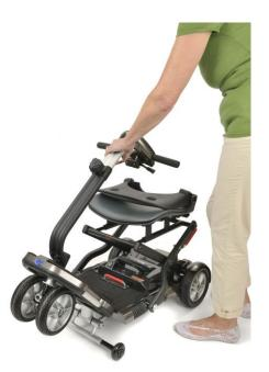
3. Ensure your Minimo Plus is locked in the unfolded position by pulling the seat away from the floor pan with one hand and pushing the tiller away from the seat with the other until you hear a click and feel you Minimo Plus lock into this position. Once your Minimo Plus is locked in position you will no longer be able to move the tiller towards and away from the seat so use this as a simple test to find out if you Minimo Plus is locked in the unfolded position.
