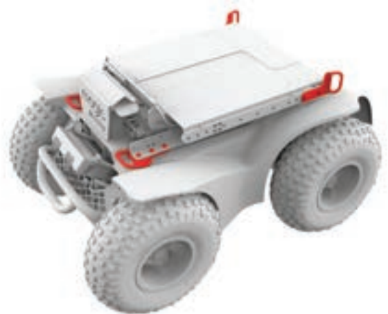
Figure 5.4d Extreme X8 tie downs
