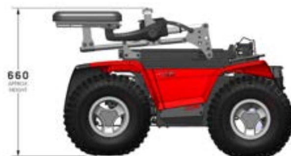
Figure 4.3f XT4 Fold Forward height
