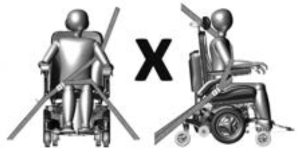
Figure 5.6 – incorrect positioning of three-point occupant restraint
