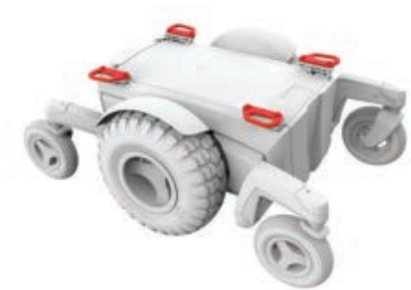
Figure 5.2a Magic 360 lifting points
