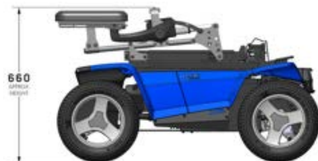
Figure 4.3e XT2 Fold Forward height
