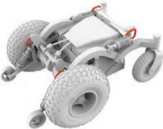
Figure 5.4c Frontier V4 tie downs
