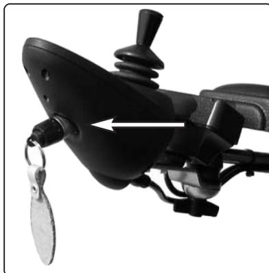
Fig.9. Panel outlet with security key
