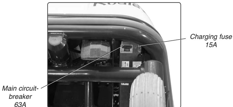
*Fig.37. Main circuit-breaker and charging fuse*
