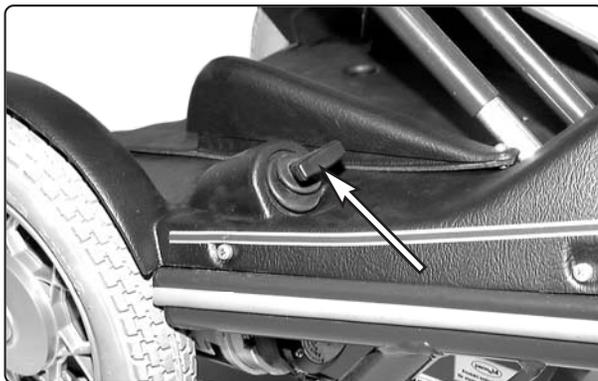
*Fig. 27. Releasing the brakes*
