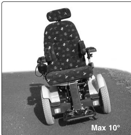
*Fig. 30. Driving along slopes*
