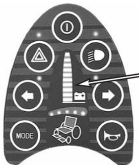
Fig.12. Battery voltage indicator
