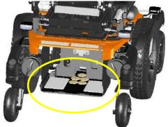
2. Two plastic spacers are to be placed in every battery box on the floor. Best is to fix them with some double sided tape.
