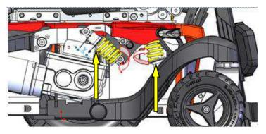
The best way is to measure the distance between the ring and the end of the tread in mm. Make sure that the spring settings in the front are identical. The same for the two rear springs.
