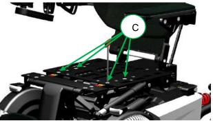
step 5: Loosen up the screws (C) of the legrest unit, using an 5mm Allen key.
