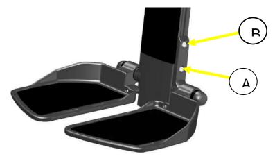
step 1: Loosen up the bottom legrest (A) bolt first, using a 5mm Allen key.
