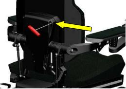
step 1: Remove the rear cover of the backrest. To do this you must use a 3mm Allen key to loosen the 6 small screws.
