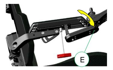
step 1: Loosen up nut (E) underneath the armrest pad using a 10mm wrench head.
