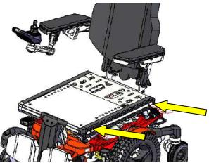
step 2: Loosen the screws of the side rail and remove them.
