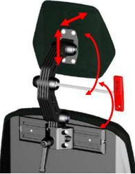
step 2: Loosen up the bolts using a 6mm Allen key. Loosen then up until the headrest can be moved.
