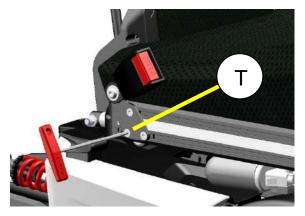
step 1: Loosen the bolts (T) using a 4mm Allen key.
