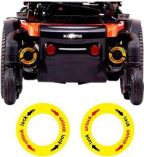
Look for the black lever on each of the driving motor locked at the rear of the chassis.
