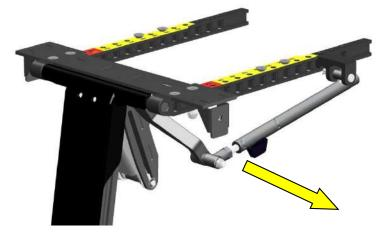
step 1: Pull the lever plate circled just enough to allow the legrest to slide.
