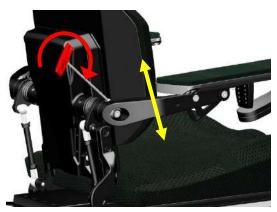
step 2: Set the armrest angle by using an 5mm Allen key. By rotating it clockwise the armrest height will increase. By rotating it counterclockwise the armrest height will be reduced.
