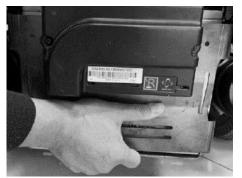
step 8. Disconnect the battery cable and then take out the battery completely to detach the positive and negative terminal. Replace the batteries.
