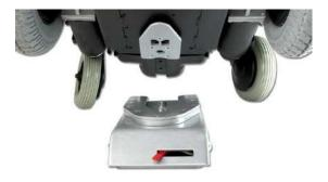
Docking station and docking plate on chassis
