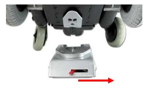
To unlock the docking station manually, the red lever needs to be pulled to the right. This retracts the locking bolt manually so the wheelchair can be released out of the docking station.
