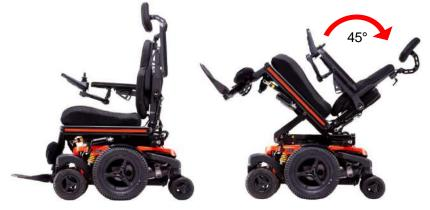
If the tilt is activated over a certain angle, the driving speed will be reduced. This is to reduce the risk of danger whilst driving at high speed.
