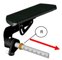
step 7: Add or remove the spacers of the axle and put the bearing back.
