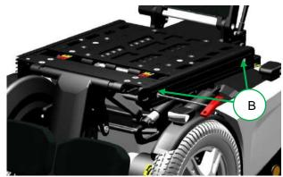
step 4: Loosen up the screws (B) of the side rails, using an Allen key size 4mm.
