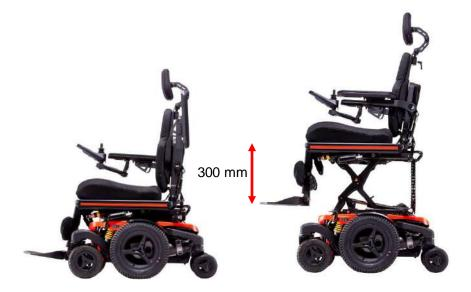
Whilst lifting the seat, the driving speed will automatically reduce to gain maximum stability at all times. At high seating position also the seat tilt will be blocked to gain maximum stability. The seat height can be set to every height position by the user. The maximum seat height is set to 760 mm (seat pan to ground)
