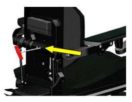
step 2: Loosen and remove the two bolts using an 5mm Allen key.
