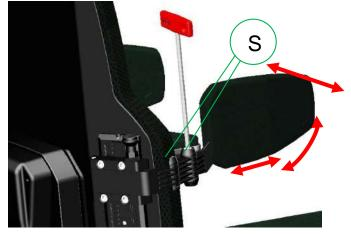
step 1: Loosen the bolts (S) of the friction joints.
