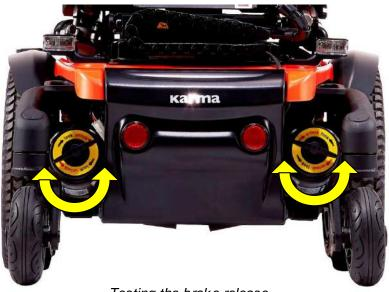
Testing the brake release
