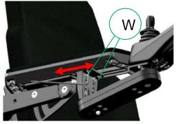
step1: Loosen the bolts (W) using a 4mm Allen key.
