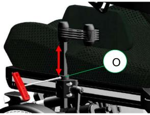
step 2: Loosen the bolt (O) of the fixation ring using a 4mm Allen key and reposition this ring against the mounting block as a stopper.
