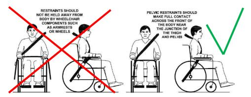
Picture of improper belt fit
