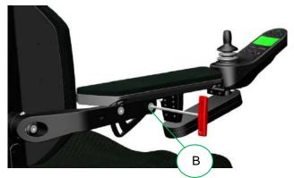
step 1: Loosen the front armrest bolt (B) using a 5mm Allen key. Don't take it out, just loosening.
