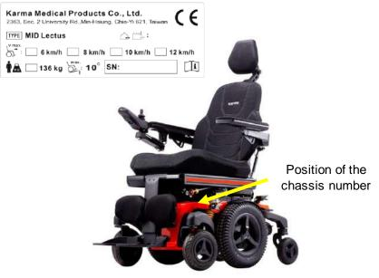
The used symbols on the chassis plate are explained below:
