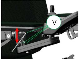
step 1: Loosen the bolts (V) using a 3mm Allen key.
