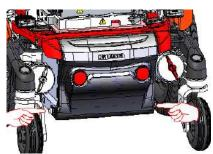
step 4. Flip up the plastic cover to detach the Velcro strip. Detach the rear covers.
