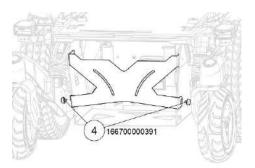
step 6. Lift up the front battery plate and then take it off.
