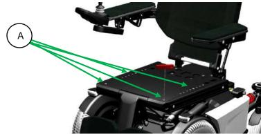
step 2: Loosen the top seat panel screws (A) using an 4 mm Allen key.
