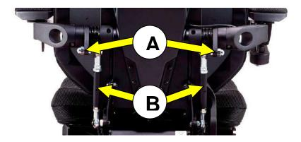
step 3: Remove the cap nut [A] and parallel bar [B] with a 12mm and 17mm open-end wrenches.
