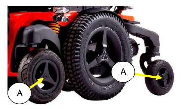
The rear- and front caster wheels should be taken off from the axle by loosening the center bolt (A).
