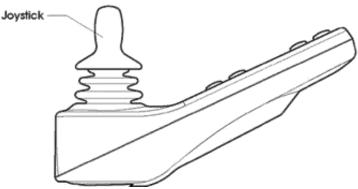
The joystick is primarily used to drive the wheelchair. Push the joystick into the direction you want to drive and the wheelchair will start to move in that direction.
