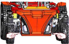
step 4. Flip up the plastic cover to detach the Velcro strip. Detach the front covers.
