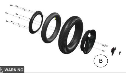
Do not loosen the central hub bolt to remove the front wheel.
