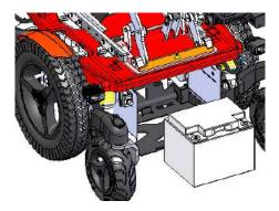
step 8. Reconnect the batteries according to the schematic which is place on the inside of the battery covers.
