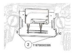
step 7. Lift up the battery plate to detach the notch and take it off.
