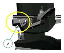
step 1: Release the locking bolts (A) on each side of the armrest using an Allen key size 5mm.
