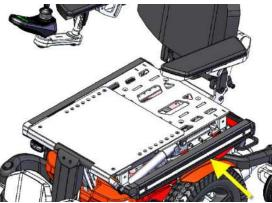
step 4: Place the extension rail in to position and place the longer mounting bolt which come with the extension rail.
