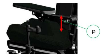
step 4: Remove the rubber covers (P) of the friction joints.
