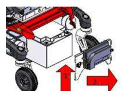
step 9. Reconnect the batteries according to the schematic which is place on the inside of the battery covers.
