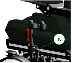
step 1: Loosen the lever knob (N) and lift up the hip support into the right height position.
