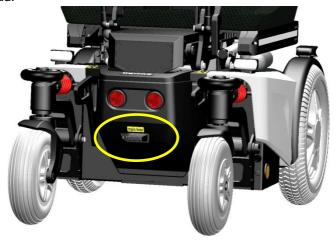
The main fuse is also used to disconnect the batteries from the electronics. This is required when transporting the wheelchair on a plane.
