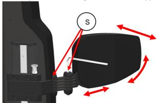
step 1: loosen the bolts (S) of the friction joints.
