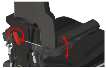
step 2: set the armrest angle by using an 5mm Allan key. By rotating it clockwise the armrest height will increase. By rotating it counterclockwise the armrest height will be reduced.
