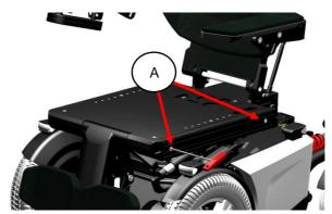
step 2: loosen the screws of the side rail (A) and remove them.
