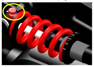
Turning the red knob clockwise (to the + direction) will reduce the movement of the piston going out again. This increases the damping of the spring damper unit. Turning the knob counter clock wise will reduce the damping. The right setting will be done by stetting and testing whilst driving.
