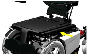
step 4: place the extension rail in to position and place the longer mounting bolt which come with the extension rail.
