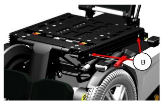
step 4: loosen up the screws (B) of the side rails, using an Allan key size 4mm.
