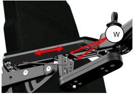
step 1: loosen the bolts (W) using a 3m Allan key.
