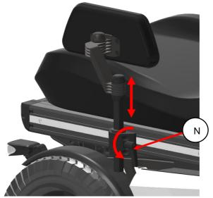
step 1: loosen the lever knob (N) and lift up the hip support into the right height position.
