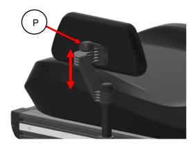
step 4: remove the rubber covers (P) of the friction joints.
