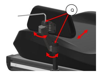
step 5: loosen the friction bolts (Q) so the padding can be moved.
