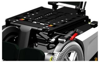
step 8: mount the side rails into position and tighten the bolts.
