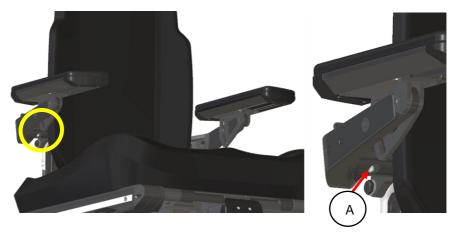
step 1: release the locking bolts (A) on each side of the armrest using an Allan key size 5mm.
