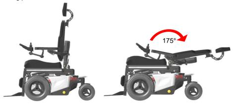
At a reclined backrest position over 135° the driving speed will be automatically reduced for safety reasons.
