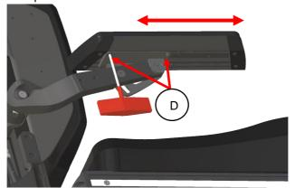
step 1: loosen up the four bolts (D) using a 3mm Allan key.
