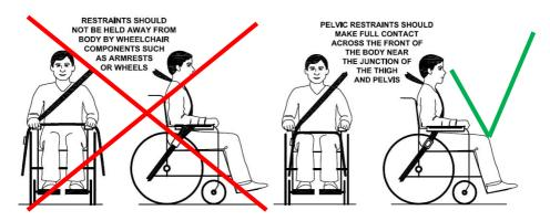
Picture of improper belt fit
