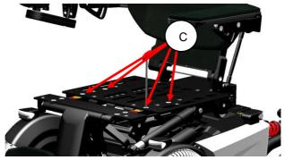
step 5: loosen up the screws (C) of the legrest unit, using an 5mm Allan key.
