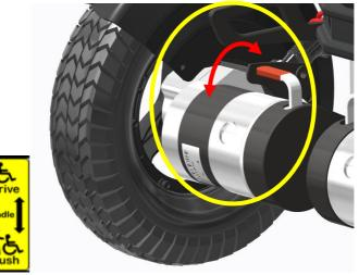
Testing the brake release
