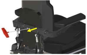
step 2: loosen and remove the two bolts using an 5mm Allan key.
