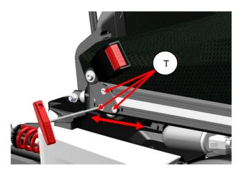
step 1: loosen the bolts (T) using a 4mm Allan key.
