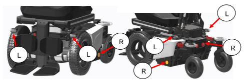
The chassis has very strong and bright LED lights to make sure you can have a safe drive in the dark. The orange reflectors on both sides and the red reflectors on the rear also make you visible for other people as well. The lights fulfill the European requirements. (E marked)
