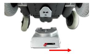
To unlock the docking station manually, the red lever needs to pull to the right. This retracts the locking bolt manually so the wheelchair can be released out of the docking station.
