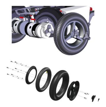
After taking the wheels of the wheelchair, the rim can be split. The tire is then available for repair. The inner tubes of the tires can be repaired according to the description on the tire puncture repair kit that you use. It is however recommended to renew the inner tube at all time when the tube has a puncture.
