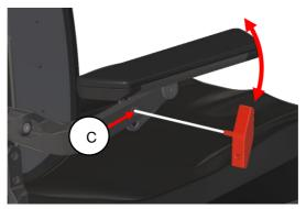
step 2: loosen up the bolt (C) slightly until the armrest starts to move.
