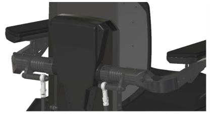
step 8: connect both parallel bars and secure them with the locking pin.
