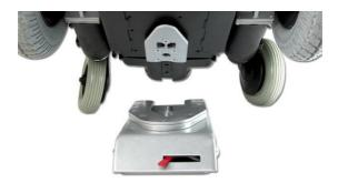
Docking station and docking plate on chassis
