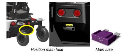
The main fuse protects the whole electrical system of the wheelchair. This fuse will only blow if there is a serious problem on the wheelchair.
