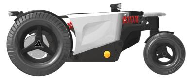
Each of the front wheels is propelled by a powerful drive motor. These motors also take care for the steering of the wheelchair. With this system it is possible to turn on the spot. This makes the wheelchair optimal for indoor use.
