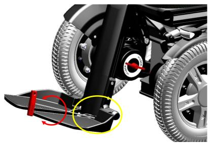
step 1: insert the 4mm Allan key into the adjustment screw inside the footplate.
