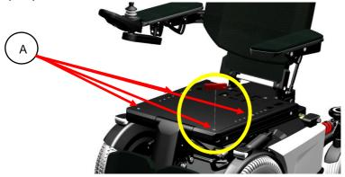
step 2: loosen the top seat panel screws (A) using an 3mm Allan key.
