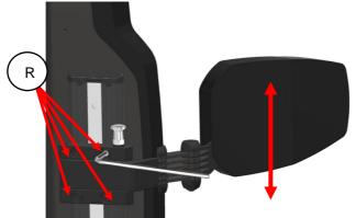
step 1: loosen up the bolts (R) using a 5mm Allan key.
