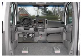
Dahl docking station mounted on the floor
