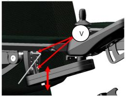
step 1: loosen the bolts (V) using a 3mm Allan key.
