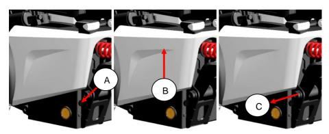
After taking the cover off, the maintenance-free battery can be pulled out of the box. Mind the cables!
