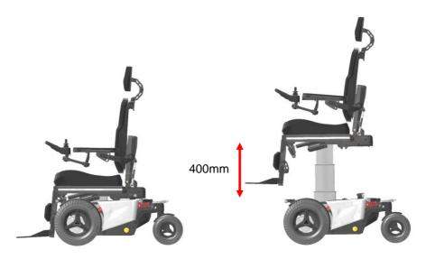
Whilst lifting the seat, the driving speed will be automatically reduced to gain maximum stability at all times. At high seating position also the seat tilt will be blocked to gain maximum stability. The seat height can be set to every height position by the user. The maximum seat height is set to 850 mm (seat pan to ground)
