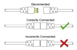
Do not hold or pull on the cable. Always grip the connector when connecting and disconnecting.
