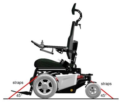
The straps must be connected to the vehicle at suitable anchor points. Make sure that the tire pressure is at the recommended level so the straps can have maximum effect. Make sure the straps are tightened to maintain optimal security.
