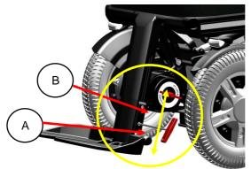
step 1: loosen up the bottom legrest (A) bolt first, using a 5mm Allan key. step 2: slowly loosen up the top end bolt (B). Just enough to feel the footplate is starting to move.
