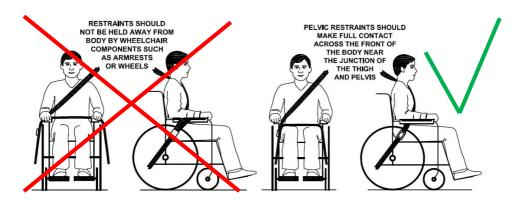
Picture of improper belt fit
