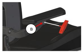
step 1: loosen the front armrest bolt (B) using a 5mm Allan key. Don't take it out, just loosening.
