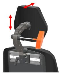
step 2: loosen up the bolts using a 6mm Allan key. Loosen then up until the headrest can be moved.
