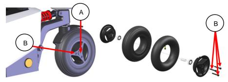
The rear wheels should be taken off from the axle by loosening the center bolt (A). The tire can be taken off by loosening the 3 bolts (B) and splitting the rim.
