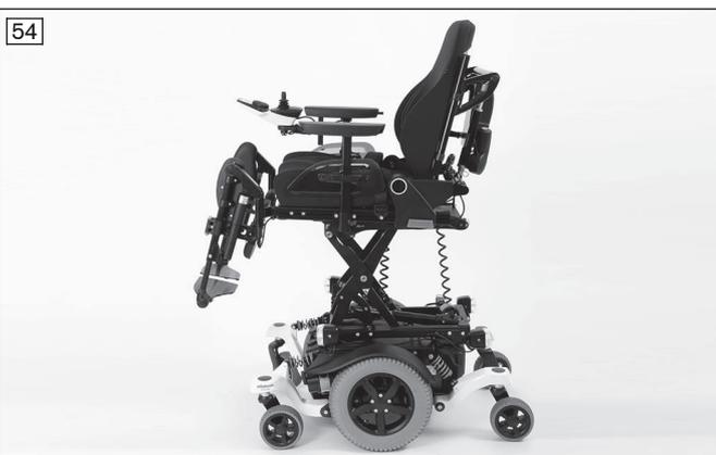
The power seat height adjustment feature raises the seat bottom by **350 mm (13.8")** using a motor drive. The seat can be moved up continuously to the height specified. The driving function can be used indoors even when the seat is raised. The speed is decreased when the seat is raised. This is indicated on the control panel as follows:
