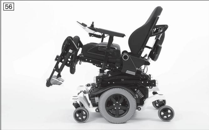
The power seat tilt function allows the seat to be tilted by up to **45°**, for example to relieve pressure (with centre of gravity shift).
