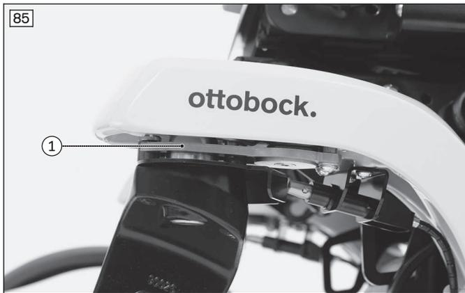
The mechanical track stabiliser (see fig. 85, item 1) under the caster wheel swing arm stabilises the caster wheels when moving forward at high speeds.
