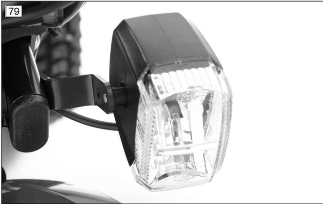
The rear lighting consists of 2 LED rear lights with integrated direction indicators.
