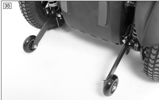
The anti-tipper makes driving safer (see fig. 35). With rear-wheel drive, it prevents the wheelchair from tipping too far backward. The anti-tipper is mounted so that the ground clearance is at least **50 mm**.
