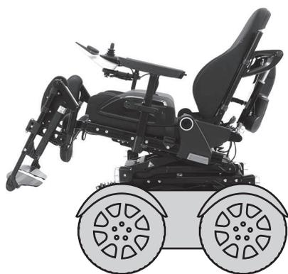
The power seat tilt function allows the seat to be tilted by up to **45°**, for example to relieve pressure (with centre of gravity shift).
