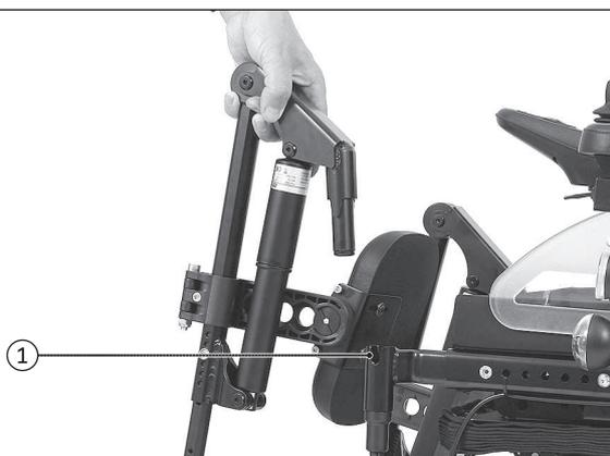
The footrests can be flipped up to increase the entry and exit area.
