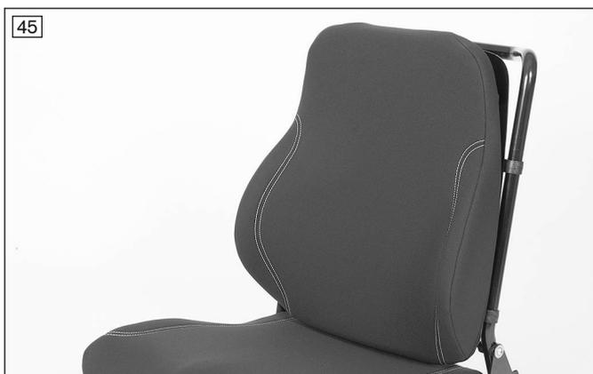
The contoured pads are offered in the flat contoured and deep contoured versions. The pads can also be covered in either cloth or artificial leather.
