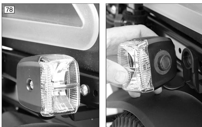
The front lighting consists of 2 front lights with integrated direction indicators (see fig. 78, left).
