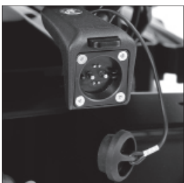
EU043 External magnetic charging receptacle
