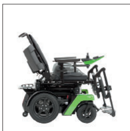
ED047 Power back support angle adjustment
