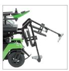
EB003 Power elevating, separate control
