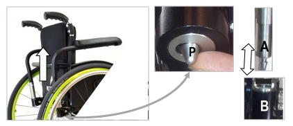
The steel support (made out of the parts A and B), does not allow the armrest to come off unintentionally. When you pull the armrest up by approximately 1 cm, it should stop at that point. In that position, as above mentioned, you can swing the armrest away.
