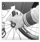
Slightly lift the wheelchair form the ground on one side by holding it on the backrest. Now one rear wheel is not touching the ground.
