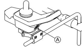
Fig. 4-11 Example of DLX-REM400 adjustment. DLX-REM110, DLX-REM211 and DLX-REM216 are adjusted the same way.
