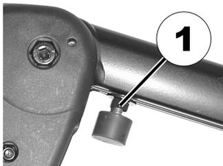
Use the wrench to loosen the counter nut (1).
