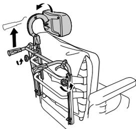
Loosen the handwheels **A** and raise the push handles as far as possible.
