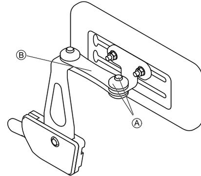
Remove upper screw and friction cap (A).
