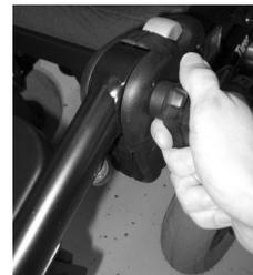
Turn the knob clockwise to tighten it.
