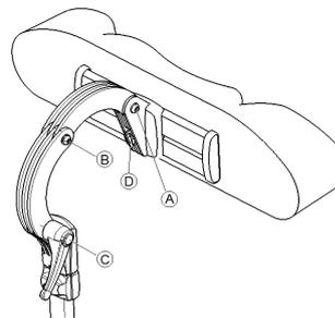
1. Loosen the screws **A** , **B** or the clamping lever **C**.
