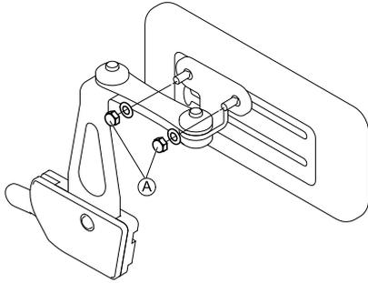
Loosen the two screws (A).
