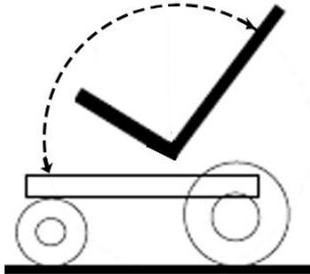
Fig. 3-5 Drive slowdown due to backrest angle
