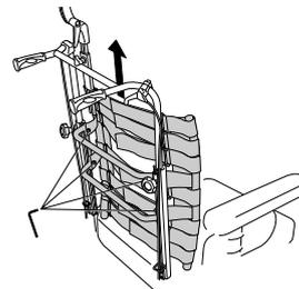
Loosen the screws **B** and remove the backrest by lifting upwards.
