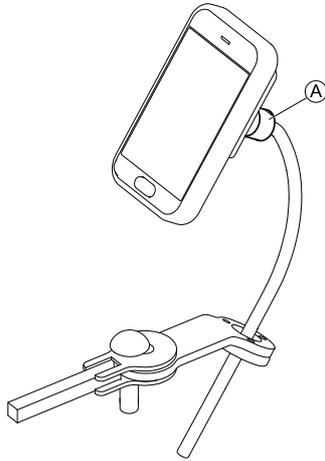
1. Loosen clamping bush (A).
