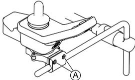
Fig. 4-10 Example of DLX-REM400 adjustment. DLX-REM110, DLX-REM211 and DLX-REM216 are adjusted the same way.
