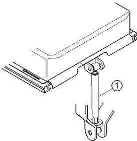
The figure shows the position of the spindle (1) for manual seat angle adjustment.
