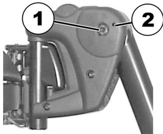
Loosen the screw (1) using the Allen key.
