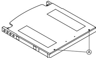
Loosen the screws (1) and remove the seat plate.
