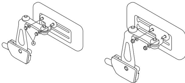
1. Loosen the two screws (A).
