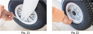
8.2.3 To replace the rear tyres, as shown in Figure 22, remove the rear wheel with the on-board tool No.5 wrench.
