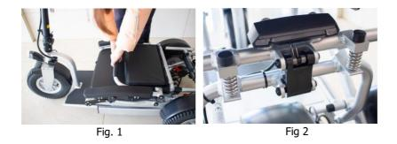
4.1.2 Folding the mobility scooter: first release the locking latch, as shown in Figure 3. With one hand to hold the backrest, the other hand to pull the seat cushion closed, as shown in Figure 4.
