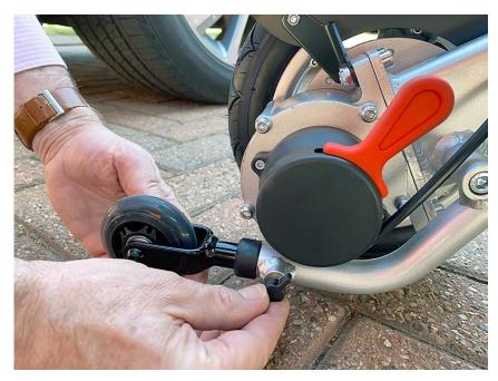
Ensure there is an anti-tip wheel fitted to each side of the chair.
