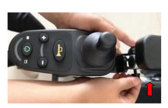
Step 2 Connecting the joystick cable
