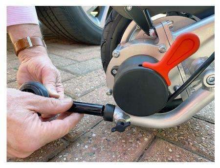
With the the wheel positioned upright as shown in the photo below, tighten the locking screw to secure the anti-tip wheel assembly inside the tube.
