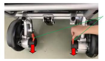
Pull back both red motor levers for normal powered mode.
