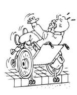
Driving over a high curb/step (more than 3cm) could result in in the chair rolling over or a serious accident.
