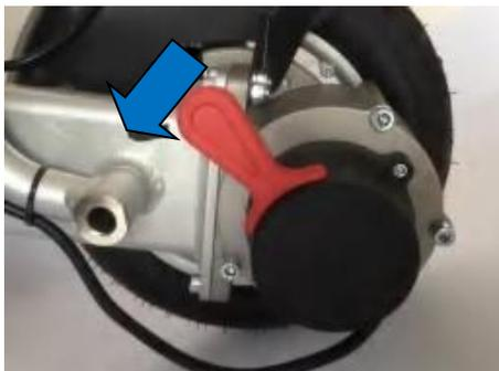
In normal powered mode, without an Attendant pushing the chair, both red motor levers should be pulled back to engage the electromagnetic brakes. Both wheels will now lock, holding the chair on the brakes.
