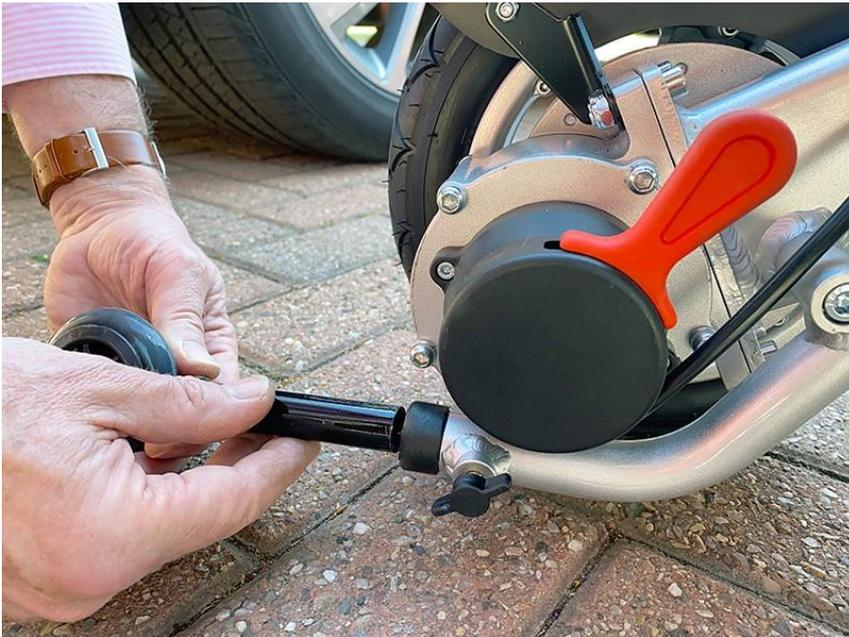
With the the wheel positioned upright as shown in the photo below, tighten the locking screw to secure the anti-tip wheel assembly inside the tube.
