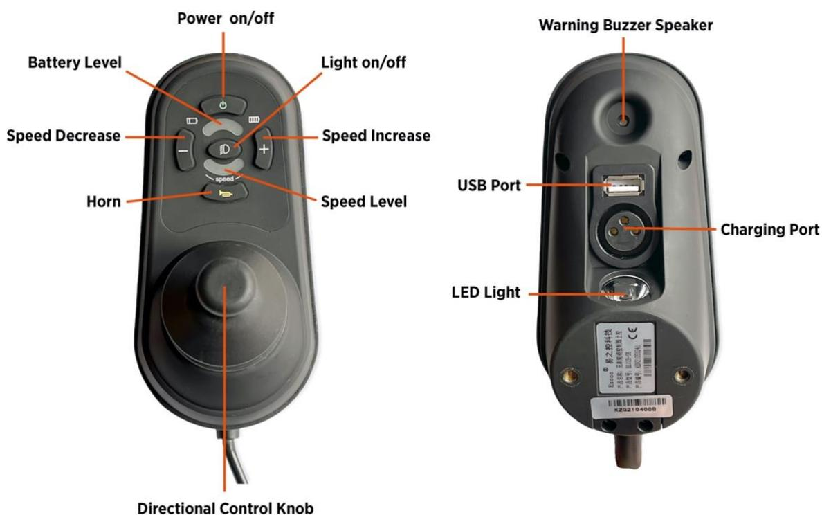
Joystick: controls the chair's direction and speed.
