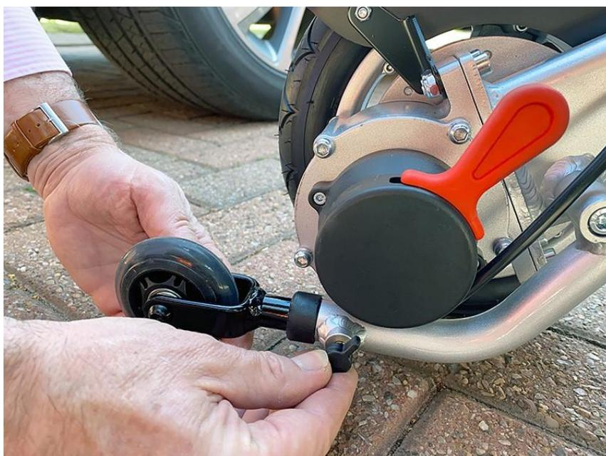
Ensure there is an anti-tip wheel fitted to each side of the chair.
