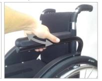
In order to check the correct position of use, with one hand, take hold of the armrest and try to move it clock and anticlockwise.
