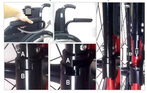
In order to check the correct position of use, with one hand, take hold of the armrest and try to move it clock and anticlockwise.
