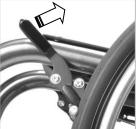
To engage the brake, push the lever forward until it locks.
