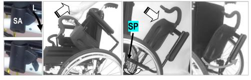
To flip the armrest up backward, lower the lever **L** of the support **SA**, then, pull it up backward. In this position, you can also turn the armrest behind the backrest pivoting it on the support **SP**.
