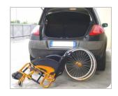
Release the brakes and remove the rear wheels.
