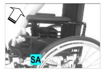
In order to check the correct position of use, with one hand, take hold of the armrest on its handhold in front and try to pull it up.
