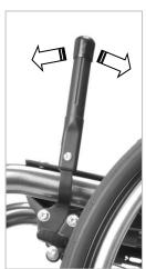
The brake (push-to-lock and pull-to-lock) with extended lever works in the same manner but results easier to engage and release.
