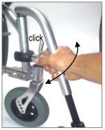
To insert the footplate frame, first lean the fork  ${\bf F}$  on the tube  ${\bf T}$ . Then, lower the footplate frame until
