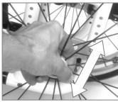
Slightly lift the wheelchair form the ground on one side by holding it on the backrest. Now one rear wheel is not touching the ground.
