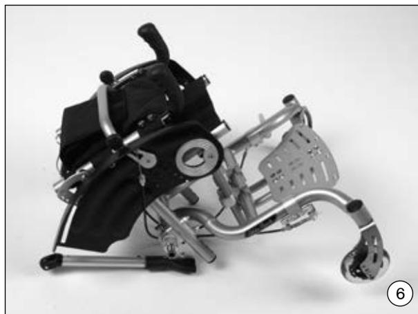
**CAUTION Risk of accident.** During assembly, it is essential to ensure that the backrest is folded back to the stop and the quick-release axles for the rear wheels are securely locked in the axle housings. It must not be possible to remove the wheel unless the button is pressed. Check the function of the wheel locks.
