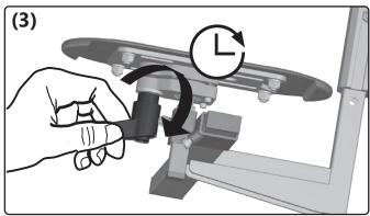
Firmly close the clamp lever and check the fixed position of the footrest.
