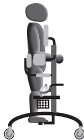
If the standing trainer is used in an area without thresholds, the wheels should be adjusted in such a way that each wheel maintains ground contact. In the case of frequent crossing of e.g. door thresholds or the like, the front wheel should not be in contact with the ground.
