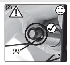
(2) After insertion, the locking ball (A) must be visibly protruding. Pull at least 1x after each insertion to test whether the quick-release axle is engaged. It should no longer be possible to pull the wheels outwards.
