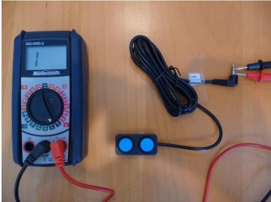
1. Without depressing any of the buttons, check for continuity between all of the 3 contacts of the mini-plug connector (1-2, 1-3, and 2-3). If there is continuity then the switch has failed.
