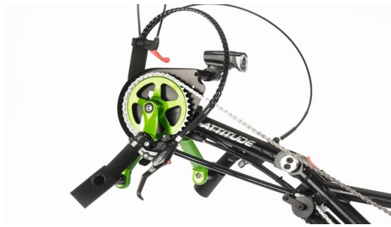
Fork for Attitude Manual & Hybrid, angle and depth-adjustability of crank-position
