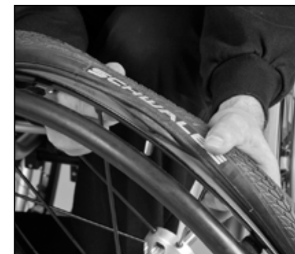
Image 62 Pull out the tube
