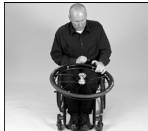
Image 61 Pull the tire edge over the rim
